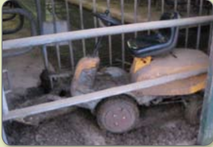
The manure can be cleaned by manure slide mounted on a mini-bulldozer.
