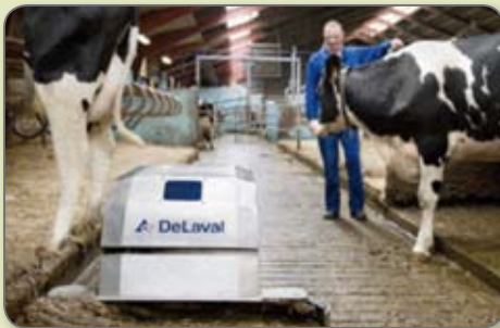
The manure can be cleaned by a robot scraper or a mobile barn cleaner. At regular intervals the robot starts automatically and follows a pre-programmed path.
