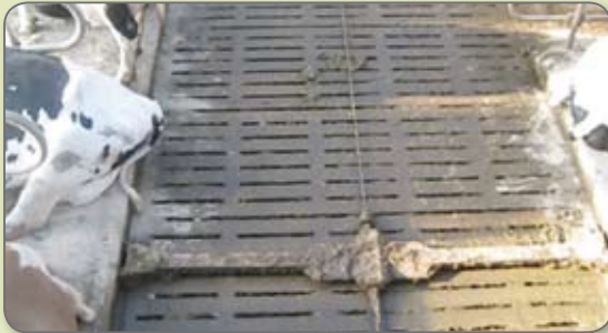
The manure can be cleaned by an electrical manure slide. This scraper moves back and forth at regular intervals.
