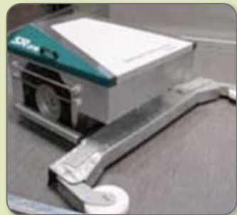
The manure can be cleaned by a robot scraper or a mobile barn cleaner. At regular intervals the robot starts automatically and follows a pre-programmed path.
