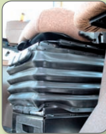
Air suspended seat than can be adjusted to the driver's size and weight.
