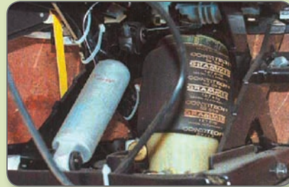
Air suspended seat than can be adjusted to the driver's size and weight.
