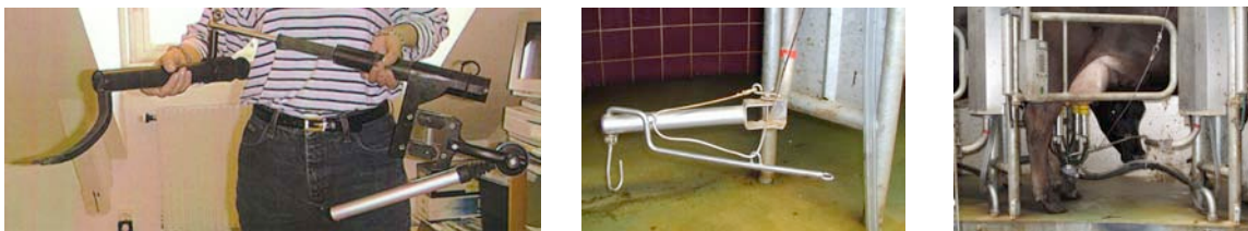
Different support arms for placing of the milking cluster
